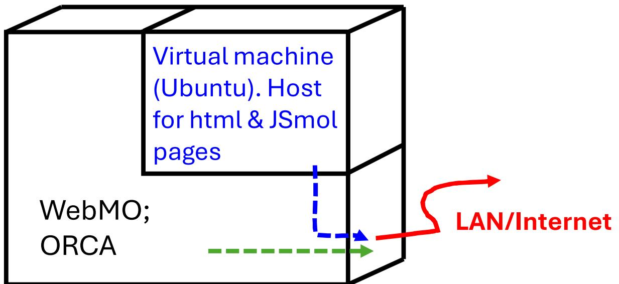
A **virtual machine** is installed on WebMO server with the two Linux OS's sharing a network interface. In my experience, the Linux/Apache instance running WebMO cannot also host a normal html websites.
